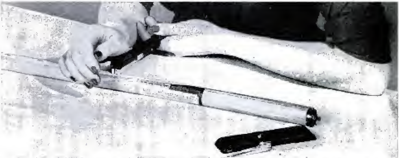
Anybody who has ever tried to tack a new shade to a roller will find the operation easier with a stapler
